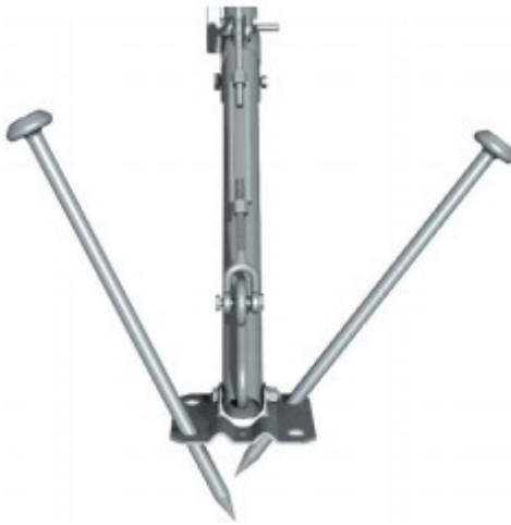
FIGURE B-2. Staking the tripod feet
